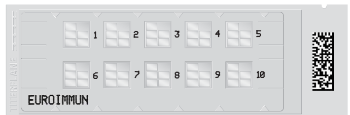
Fig.: Mouse Monitoring Mosaic slides with BIOCHIP mosaic: Each BIOCHIP is coated with one cell line infected with a specific virus type. Further substrates for the health monitoring of laboratory mice are available and can be used for the preparation of customer-specific mosaics.
